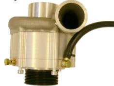
With the supercharger properly in place fit one end of the hose to the oil inlet using the banjo fitting and banjo bolt. Make sure to use a copper washer on each side of the banjo fitting to prevent leaks
