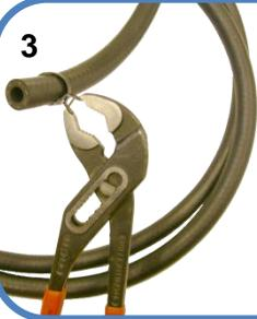
With a pair of pliers, compress a hose clamp and slide it over one end of the hose. Press a banjo fitting into the hose end and secure it with the hose clamp
