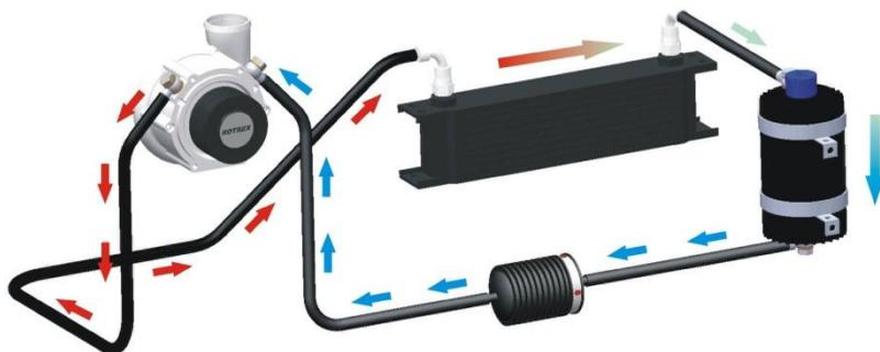
The finished oil system is shown above with oil flow direction as indicated by the arrows. Oil flows from the oil canister through the filter into the compressor oil inlet. The compressor oil outlet routes through the cooler before entering the oil canister at the top.
