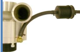
Now press the filter studs into the hose ends as shown and secure with hose clamps. Observe the flow direction of the filter! Following the same method, continue fitting the remaining part of the oil system
