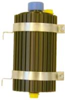
Place the oil canister with the cap **below or level** with the supercharger's shaft. Use the bracket supplied in the oil set. Make sure the canister is placed upright. Leave the plastic plugs in place to prevent debris from entering the system
